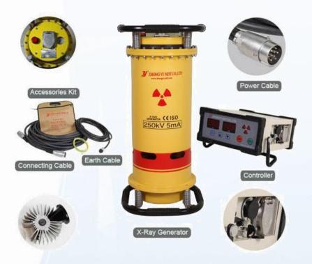
Portable NDT x ray machine is used for inspect the inner fault of the material. It adopts radiography theory to make the image on the film, in order to evaluate the work piece.
