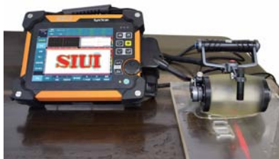
Linear Scan Image on Flat Panel Engraved with SIUI logo.
