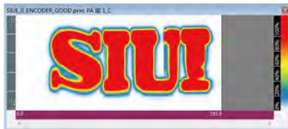
C Scan In-Amplitude, showing echo amplitude
