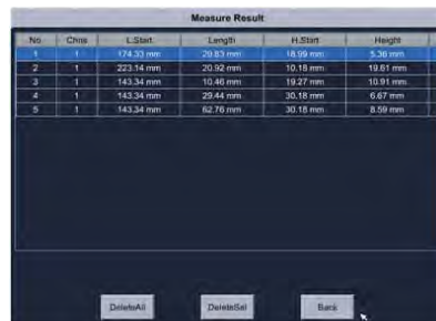
TOFD Measurement Result
