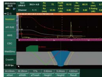
Crack Height Measurement
